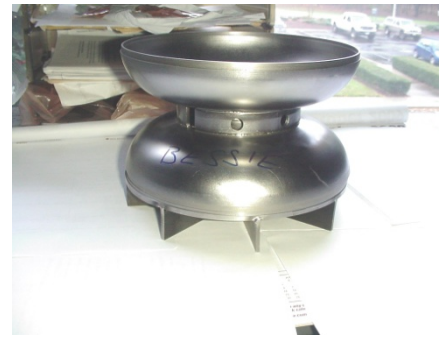
Large grain cavity backwall for cathode
