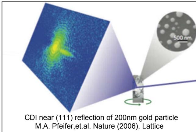
Coherent diffraction imaging (CDI) of nanoscale strain has wide application for understanding nanomaterials under extreme pressure & temperature, and during deformation or chemical processing. X-ray methods are especially suited for in-situ measurement for example inside a diamond anvil cell (DAC).
