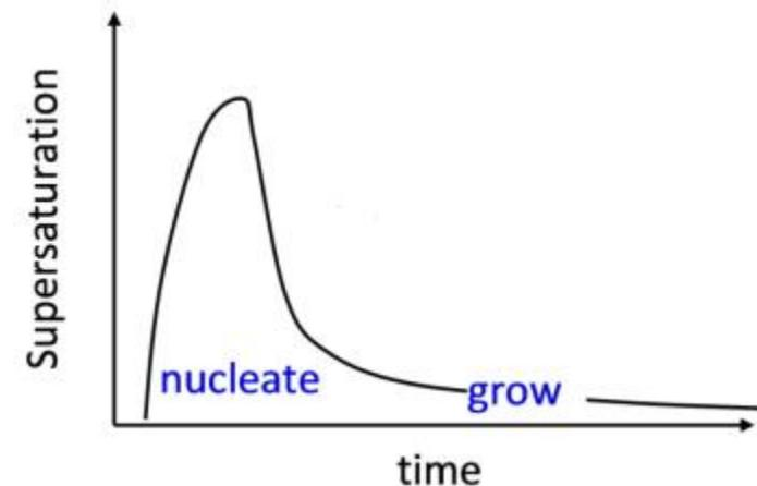
XOp microfluidic chip optimizes crystal growth by varying the degree of supersaturation versus time. See [www.elsie.brandeis.edu](http://www.elsie.brandeis.edu); Shim et al., JACS 127 (2007) 8825.
