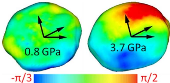
*Upper left illustration: CDI experiment and representative data. Lower left: Phase retrieval methods can produce 3-dimensional strain maps - color represents atomic scale lattice strain along specific directions resulting from pressures & surface truncation.*
