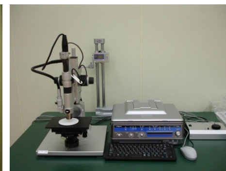
3D inspection equipment for Nb surface
