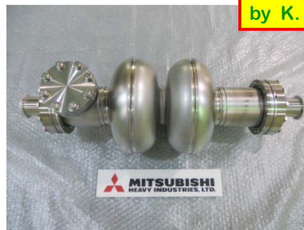
MHI-B 2-cell cavity (seamless dumbbell)
