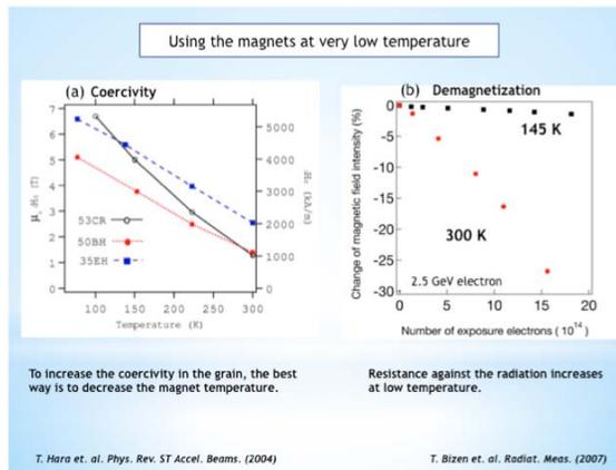
Figure 9: To increase the coercivity in the grain, the best way is to decrease the magnet temperature. (a) The coercivity increases with the temperature decrease. (b) Resistance against the radiation remarkably increases at low temperature.
