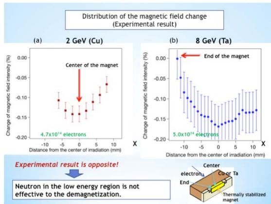
Figure 7: The experimental results of the distribution of the magnetic field change. The demagnetization shows opposite of the calculation result. Little demagnetization is shown at the end of the thermally stabilized magnet irradiated with an 8 GeV electrons to the tantalum target. This discrepancy implies that the neutron in the low energy region is not effective to the demagnetization.
