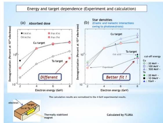
Figure 8: Comparison between the calculations and the experimental results of the demagnetization irradiated with different energy of electrons. The calculation results are normalized to the 4 GeV experimental results. (a): The absorbed dose: Experimental result of the tantalum target is different from calculation. (b): The star densities: Both experimental results of copper and tantalum target are better fit to the calculation.
