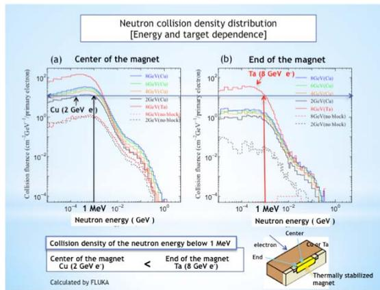
Figure 6: Calculated neutron collision density distribution. In the neutron energy below 1 MeV, the collision density at the center of the magnet irradiated with a 2 GeV electrons to the copper target is smaller than that at the end of the magnet with an 8 GeV to the tantalum target.
