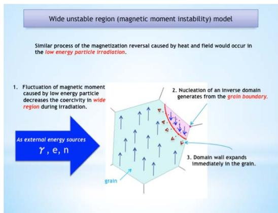
Figure 2: Wide unstable region model. Energy of  $\gamma$ ,  $e$  and  $n$  is transferred in long range to the magnet atoms as ionization and excitation. This causes the instability of the magnetic spin in the region of over the grain size. Similar process of the magnetization reversal caused by heat and field occurs by radiation.
