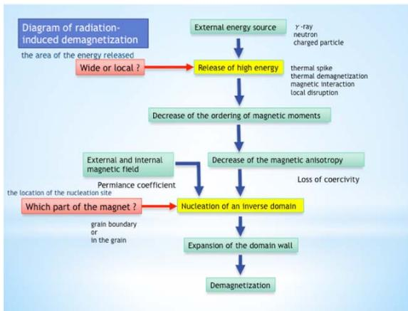
Figure 1: Diagram of the process of the radiation-induced demagnetization.
