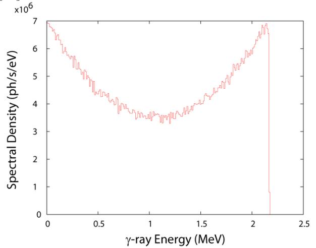
Figure 3: Calculated  $\gamma$ -ray spectrum for the high-flux mode of the designed ERL  $\gamma$ -ray source. The total flux is  $1.0 \times 10^{13}$  ph/s.
