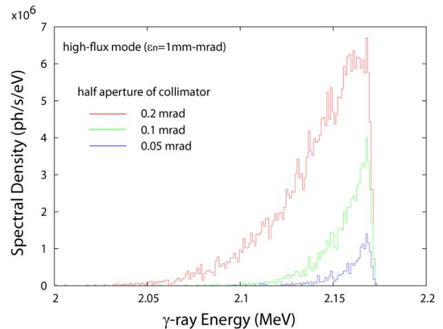
Figure 4: Calculated  $\gamma$ -ray spectrum for the high-flux mode with various sizes of on-axis collimators. Collimator half aperture is  $0.2\text{ mrad}$ ,  $0.1\text{ mrad}$  and  $0.05\text{ mrad}$ .
