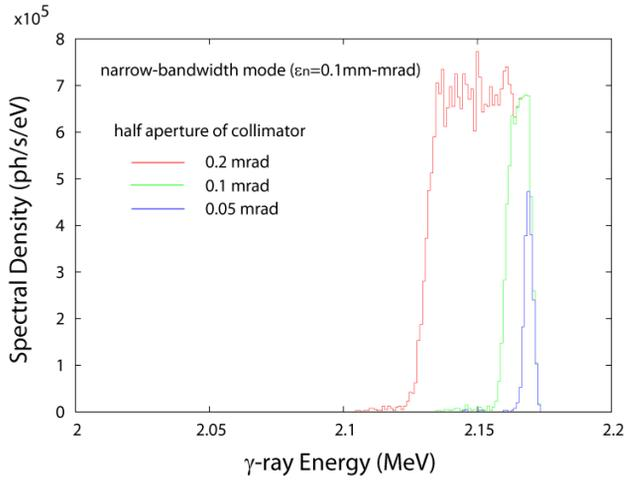
Figure 5: Calculated  $\gamma$ -ray spectrum for the narrow-bandwidth mode with various sizes of on-axis collimators. Collimator half aperture is 0.2 mrad, 0.1 mrad and 0.05 mrad.
