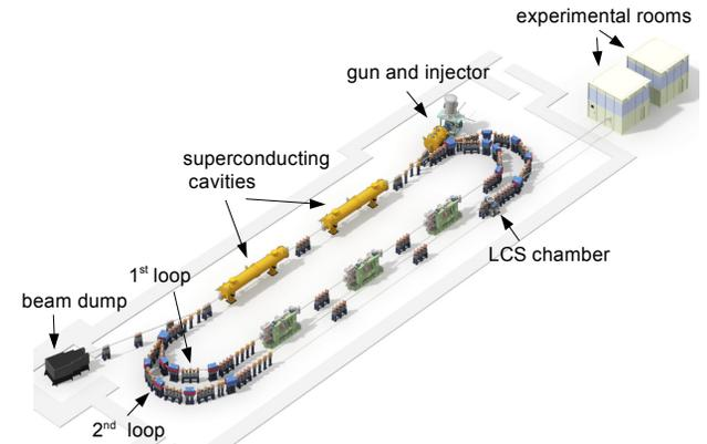
Figure 6: A schematic view of the LCS  $\gamma$ -ray experiment at the Compact ERL.
