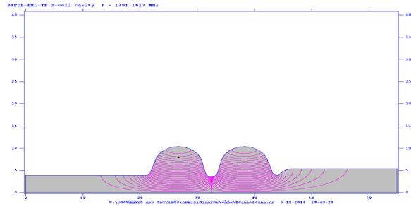
Figure 4: Electric field distribution in 2-cell cavity.
