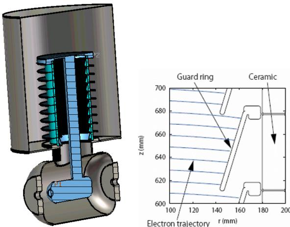
Figure 3: DC gun with segmented insulators (left) and guard rings(right).
