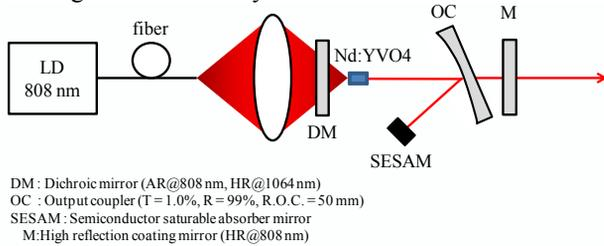
Figure 8: Schematic of Nd:YVO<sub>4</sub> oscillator.
