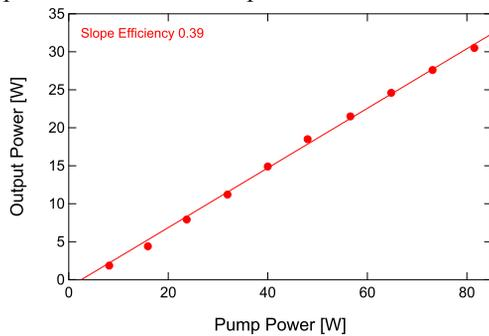
Figure 3: Amplifier slope efficiency.
