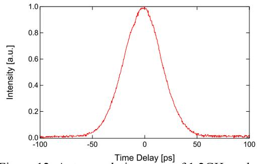
Figure 12: Autocorrelation trace of 1.2GHz pulse.
