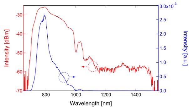
Figure 7: Spectrum of supercontinuum light.
