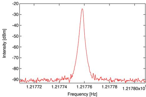
Figure 9: RF spectrum of Nd:YVO<sub>4</sub> oscillator pulse.
