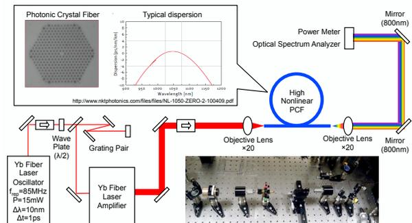
Figure 6: Setup of supercontinuum generation.
