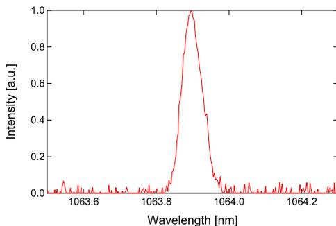
Figure 11: Optical spectrum of 1.2GHz pulse.
