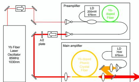
Figure 2: Schematic of Yb fiber laser amplifier system.
