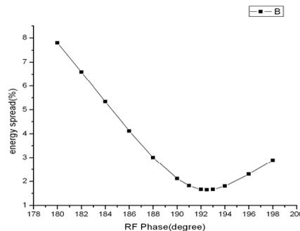
Figure 5: Energy spread after deceleration as a function of the phase in the linac.
