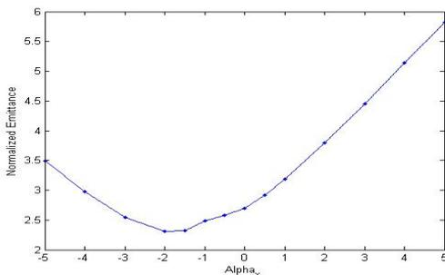
Figure 3: Normalized emittance at the entrance of the undulator.
