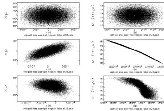
Figure 4: Beam distributions in the x and t phase space. The upper figures is taken at the entrance of Merger, the middle figures at the entrance of the first arc while lower ones at the entrance of the undulator.
