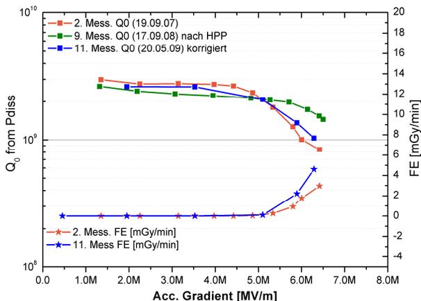
Figure 14. Unloaded quality factor  $Q_0$  vs. acceleration gradient and the corresponding field emission dose (right side). “2.Meas” taken September 2007, “9.Meas” taken after high power RF processing (HPP) of the cavity in September 200; “11.Meas” taken after reinstallation in spring 2009.
