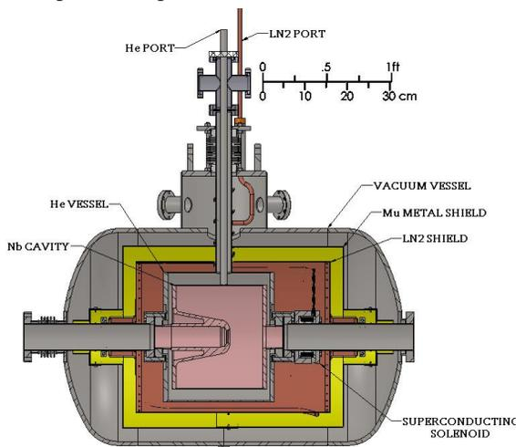
Figure 8. NPS 500 MHz superconducting gun cryomodule
