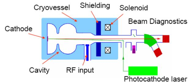
Figure 4. The HZB 1 1/2 cell 1.3 GHz photoinjector layout schematic.
