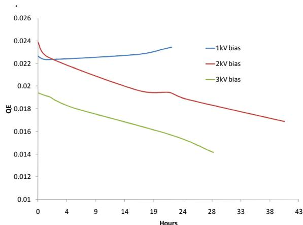
Figure 2: QE decay w/  $1.3 \text{ mA/mm}^2$  current density.
