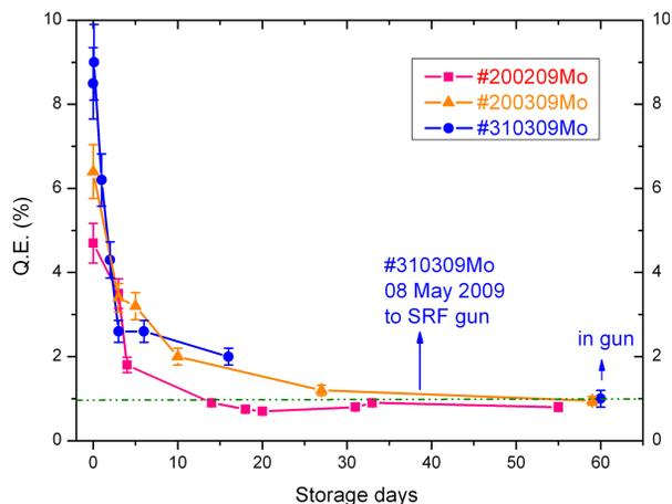
Figure 13. Long-term behavior of Cs<sub>2</sub>Te photo cathodes for the SRF gun.
