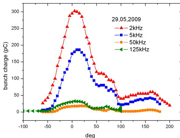
Figure 15. Laser phase scan with 55 mW laser power for different laser pulse repetition rates.
