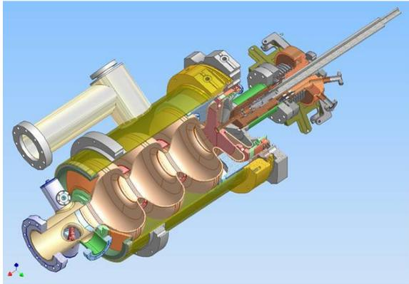
Figure 3. The FZD 3 1/2 cell 1.3 GHz photoinjector.
