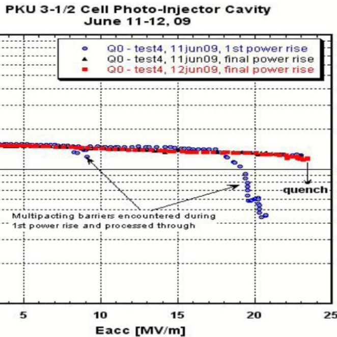
Figure 10. Vertical test result of 3.5 cell large grain Nb cavity
