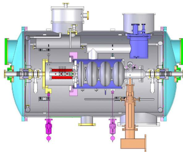
Figure 9. Schematic of 3+1/2 cavity DC-SRF injector
