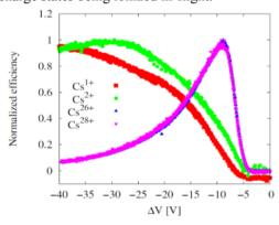
Figure 14: Relative efficiencies for cesium charge breeding as a function of the DeltaV.
