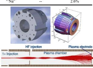
Figure 10: Symmetrized injection magnetic plug and its RADIA model, SIMION 3D trajectories.
