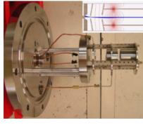
Figure 12: LPSC ion gun with its extraction optics.
