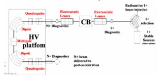
Figure 2: Scheme of the charge breeding part of SPES
