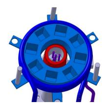
Figure 3: Mechanical design of the hot COMIC source, purple: HF couplers, red: hot plasma cavity, blue: water cooled magnets support
