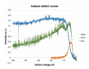
Figure 15: Relative efficiencies for sodium charge breeding as a function of the DeltaV
