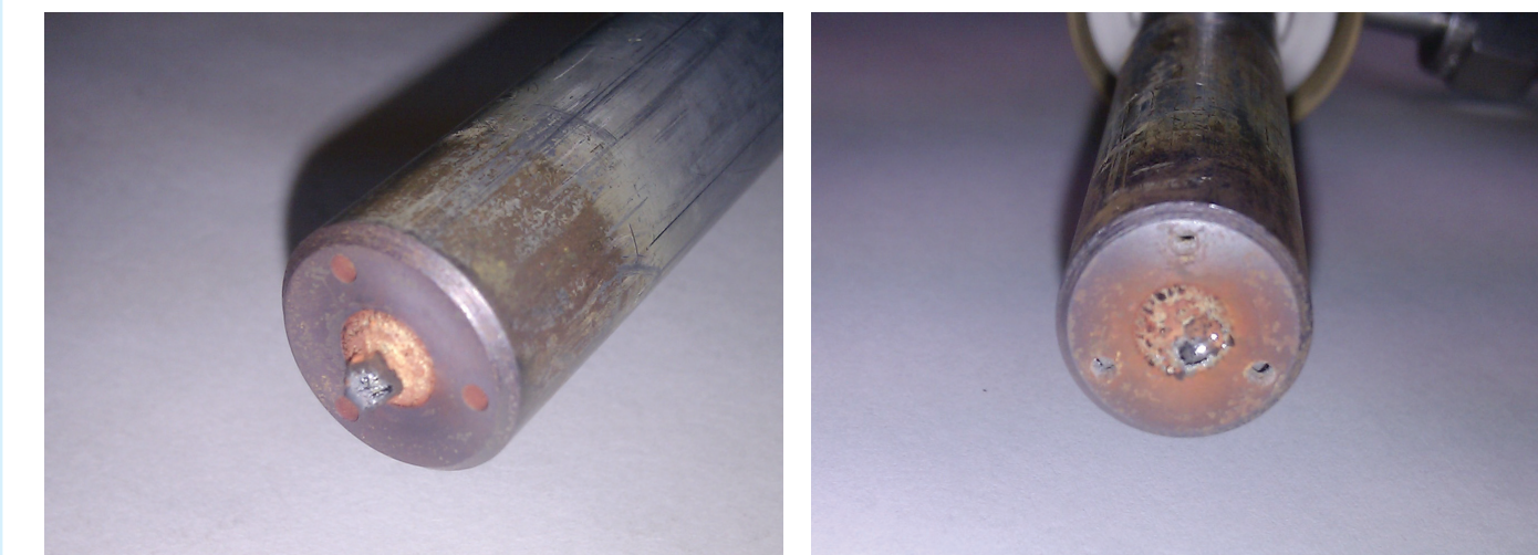
Oven tip after 2 weeks operation (normal filling and filling with liquid lead).
