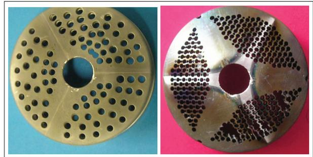
Figure 5: Extraction electrode with additional holes for pumping. No additional load for the extraction power supply caused by these additional holes has been observed (left). In case the plasma electrode is not aligned to the hexapolar pattern additional current load has been observed (right)[9].
