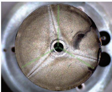
Figure 6: Sputter marks observed on the inner side of the plasma electrode. The tilt angle is  $\approx 13^\circ$  counter clockwise in relation to the vertical plane. This is in good agreement with the values for the original orientations calculated in table 1.
