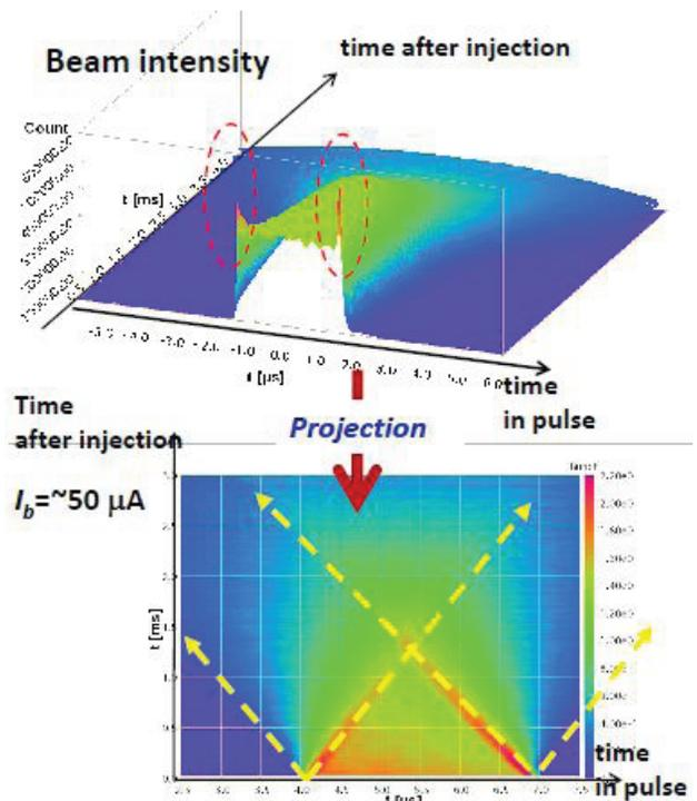
Figure 10: Mountain view of the freely circulating chopped pulse (top) and its projection on the time-turn plane (bottom).
