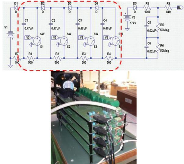
Figure 6: Equivalent circuit of the Marx generator and its photo.
