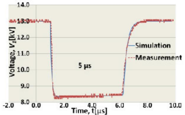
Figure 7: Pulse voltage for chopper performance.
