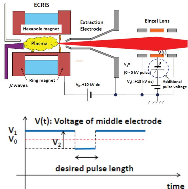
Figure 3: Idea of the Einzel lens chopper (upper) and Voltage profile of the Einzel lens  $V(t)$  (bottom).
