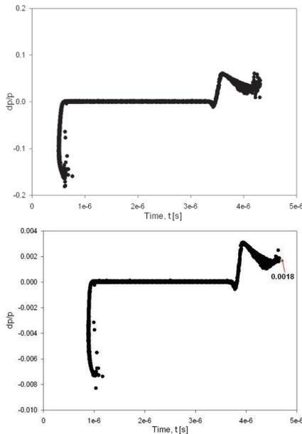
Figure 11: Phase space plot just after the Einzel lens (top) and the post acceleration column (bottom), where a relative momentum deviation is largely reduced due to acceleration from 10 keV to 200 keV,  $(\Delta p/p) = (-0.16)(10\text{keV}/200\text{keV}) = -0.008$ .
