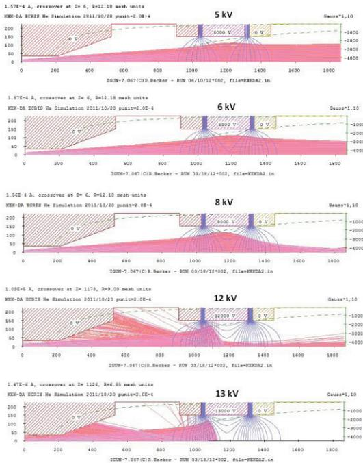
Figure 4: IGUN simulations for different Einzel lens voltages.
