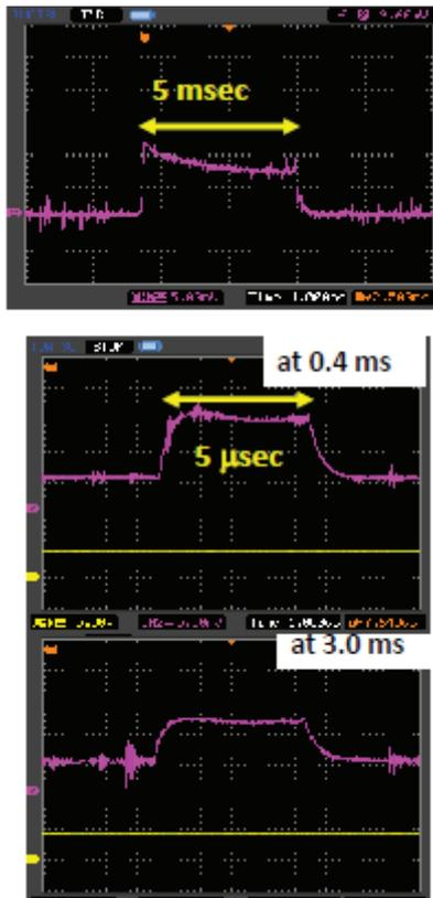
Figure 8: 5  $\mu\text{s}$  chopped pulse profiles, which are chopped at different times from the pulse head of a 5 ms ion pulse.
