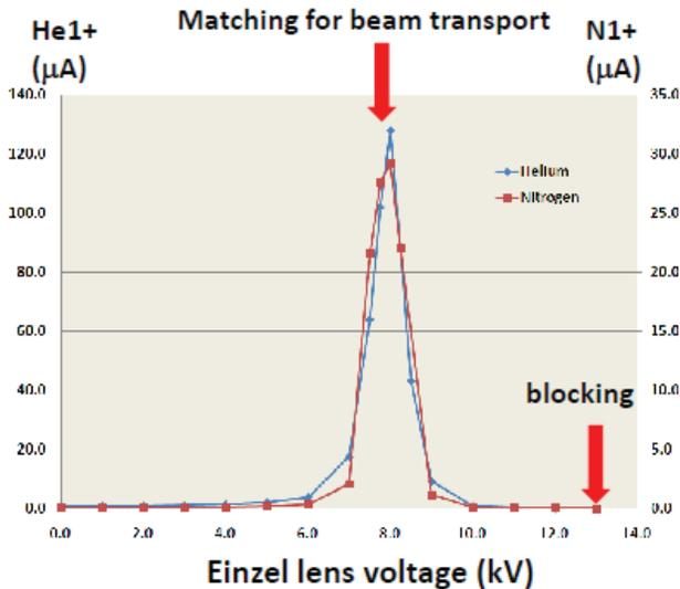
Figure 5: Beam Current for He1+ and N1+ vs. Einzel lens voltage.
