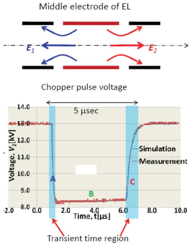
Figure 12: Model of the EL (top) and Typical chopper pulse with transient regions (bottom).
