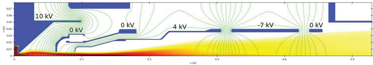
Figure 2: Simulation result (logarithmic trajectory density) for the old extraction system with 1 mA of argon beam, charge states  $1+ \dots 16+$ , tuned for optimum performance. From left to right, plasma electrode (10 kV), puller electrode (0 kV), grounded puller holder, deceleration electrode (4 kV), Einzel electrode (-7 kV) and Einzel ground electrode.
