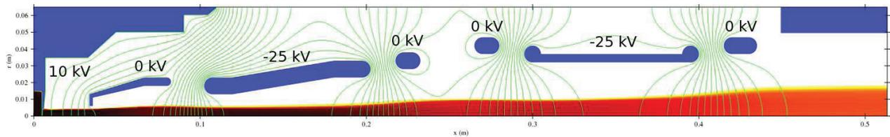
Figure 4: Simulation result for the new extraction system with 1.5 mA of argon beam, charge states  $1+ \dots 16+$ , tuned for optimum performance. From left to right, plasma electrode (10 kV), puller electrode (0 kV), first Einzel (-25 kV), Einzel lens ground electrodes, second Einzel (-25 kV) and Einzel ground electrode.
