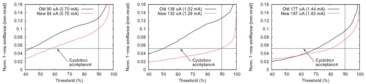
Figure 7: Emittance threshold analysis of  $^{40}\text{Ar}^{8+}$  for various beam currents. Total extracted current in parenthesis. The 90 % threshold value, used for emittance comparisons, and the K-130 cyclotron acceptance (0.052 mm mrad) are indicated with dashed lines.
