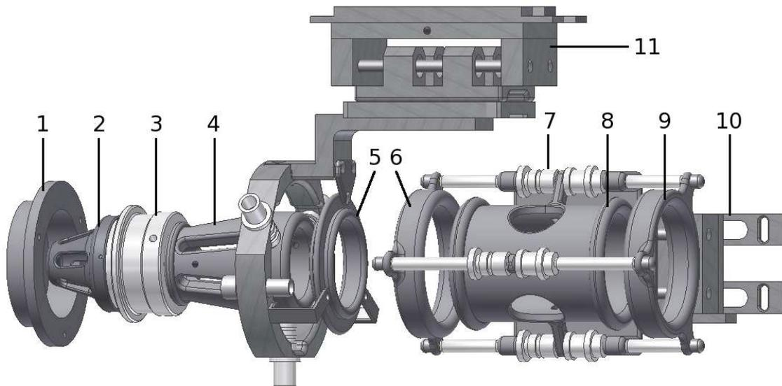
Figure 6: The new extraction system with a plasma electrode (1), a puller electrode (2) and two Einzel lenses (2-5 and 6-9). Macor and alumina are used as insulating materials (e.g. 3, 7). Lense positions can be varied independently (10, 11).
