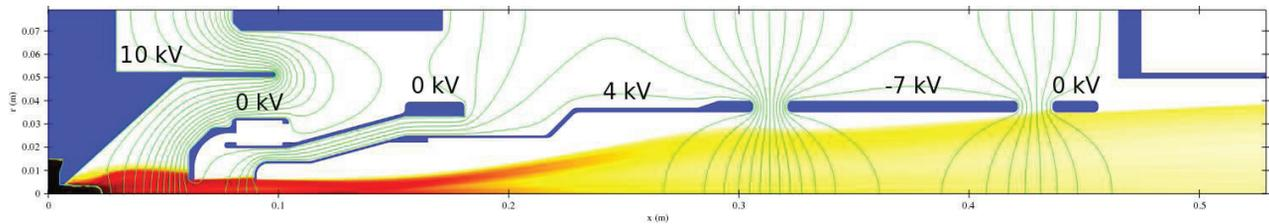
Figure 3: Simulation result for the old extraction system with 3.0 mA of argon beam with same settings as in Fig. 2. Varying electrode voltages shifts beam losses between electrodes, leading no insignificant improvements in the extracted beam.
