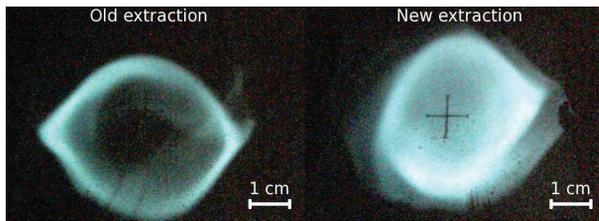
Figure 8:  $^{40}\text{Ar}^{8+}$  profiles measured after mass separation with old and new extraction designs. Total extracted beam  $\sim 1$  mA and mass separated beam current  $\sim 130 \mu\text{A}$  in both cases.
