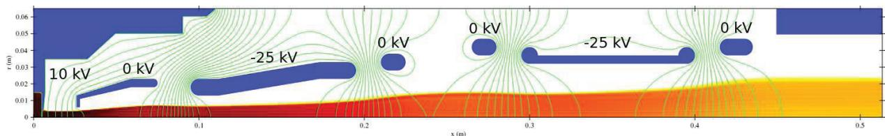
Figure 5: Simulation result for the new extraction system with 3 mA of argon beam with same settings as in Fig. 4.
