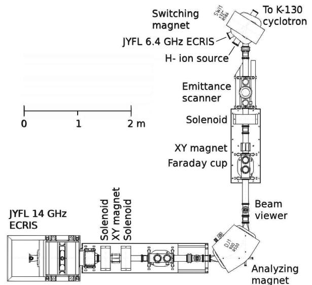
Figure 1: First section of the JYFL LEBT beginning from the JYFL 14 GHz ECRIS.
