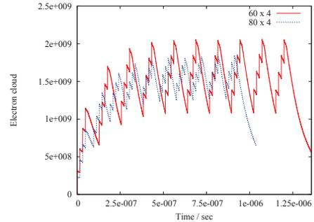
Figure 23: Simulation of electron cloud build-up for a  $60 \times 4$  and  $80 \times 4$  bunch filling and bunch population of  $1.0 \cdot 10^{10}$  and  $0.75 \cdot 10^{10}$  (SEY:  $\delta_{max} = 2.5$ )
