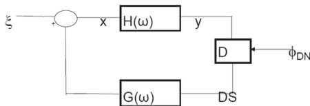
Figure 2: Schematic layout of the PETRA III feedback system [5]: The beam dynamics is described by  $H(\omega)$  and the feedback effect by  $G(\omega)$  acting on external disturbances of the beam  $\xi$ .  $\Phi_{DN}$  is the noise associated with the feedback detector D.
