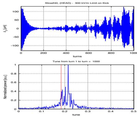
Figure 10: Vertical displacement vs. turns and fractional tune of a slice in the head of the bunch. The kicker signal saturates at  $2.874 \cdot 10^{-5}$  eV.sec/m. The beam becomes increasingly unstable and the fractional tune maximum peak is shifted to  $[Q_y] = 0.2152$ .
