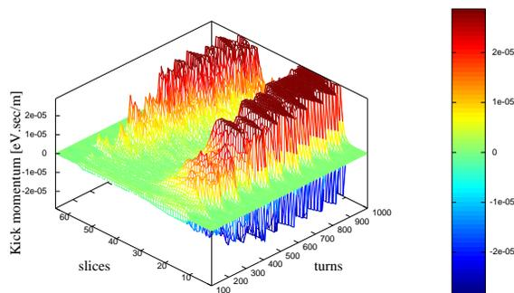
Figure 8: Momentum, slices vs. turns, applied to the bunch by the kicker, the signal is set to saturate at  $2.874 \cdot 10^{-5}$  eV.sec/m. Slices close to 0 are in the tail of the bunch, while slices close to 64 are in the head.
