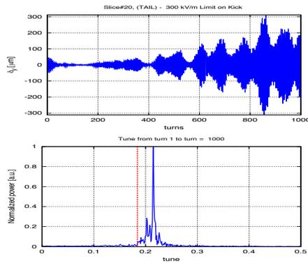
Figure 9: Vertical displacement vs. turns and fractional tune of a slice in the Tail of the bunch. The kicker signal saturates at  $2.874 \cdot 10^{-5}$  eV.sec/m. The instability grows larger and faster compared to the head. The tune is shifted to  $[Q_y] = 0.2152$ .
