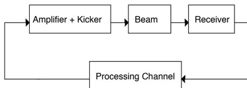
Figure 1: General scheme of the SPS Ecloud Feedback Control System.
