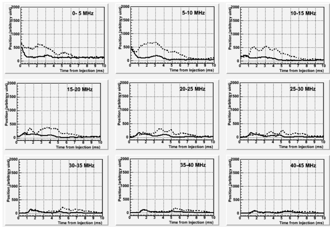
Figure 2: Time dependence of the horizontal oscillation amplitude within 10 ms from the injection for each frequency component obtained by the stripline monitor ( $\xi = -5.8$ , 130 kW). The dot lines show the case without the feedback and the solid line show the case with the feedback.
