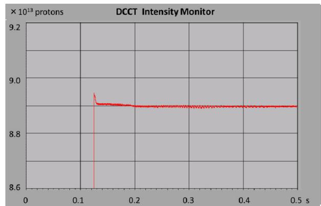
Figure 7: The beam intensity measured by the DCCT monitor with the feedback. The horizontal axis shows time from the injection.
