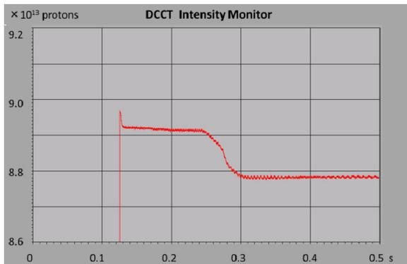
Figure 6: The beam intensity measured by the DCCT monitor without the feedback. The horizontal axis shows time from the injection.
