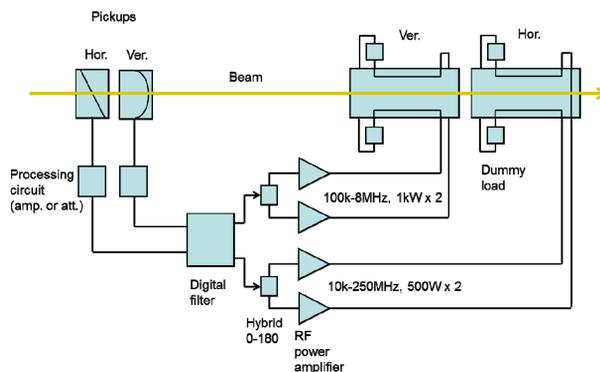
Figure 1: The schematic view of the MR transverse bunch by bunch feedback system.
