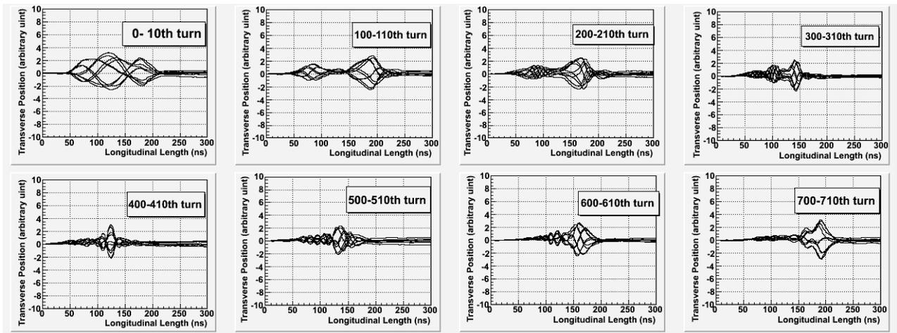
Figure 3: Transverse position depending on the longitudinal position in single bunch. The interval between each plot is 100 turns (1 turn is corresponding to about 5 microseconds) and the shapes of 10 continuous turns are superposed in each plot ( $\xi=-5.8$ , feedback on, 145 kW).
