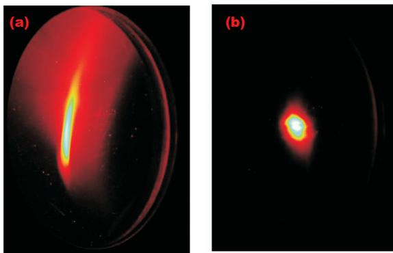
Figure 2: Dark current image on the YAG:Ce screen at 15.9 MV/m (a) and electron beam image (b).
