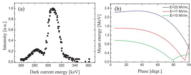
Figure 5: Dark current energy spectrum (a) and beam energy as a function of phase (b).
