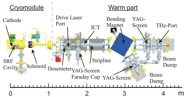
Figure 1: Schematic view of the diagnostics beam line for Stage A.
