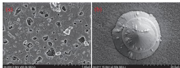
Figure 4: SEM pictures of lead deposited on optical polished niobium substrate with average roughness of 8-10 nm; 1  $\mu\text{m}$  scale (a) and 20  $\mu\text{m}$  scale (b).
