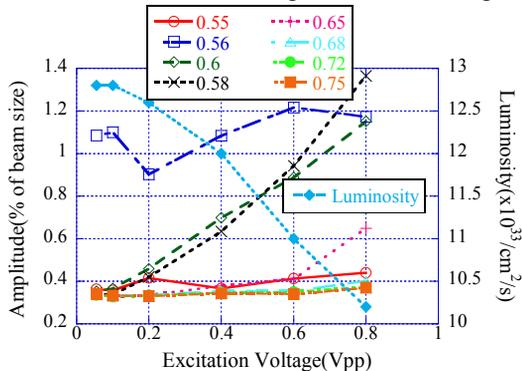
Figure 6: Luminosity response with band-limited white noise excitation. The luminosity had dropped 5% with the noise of 0.4Vpp level.
