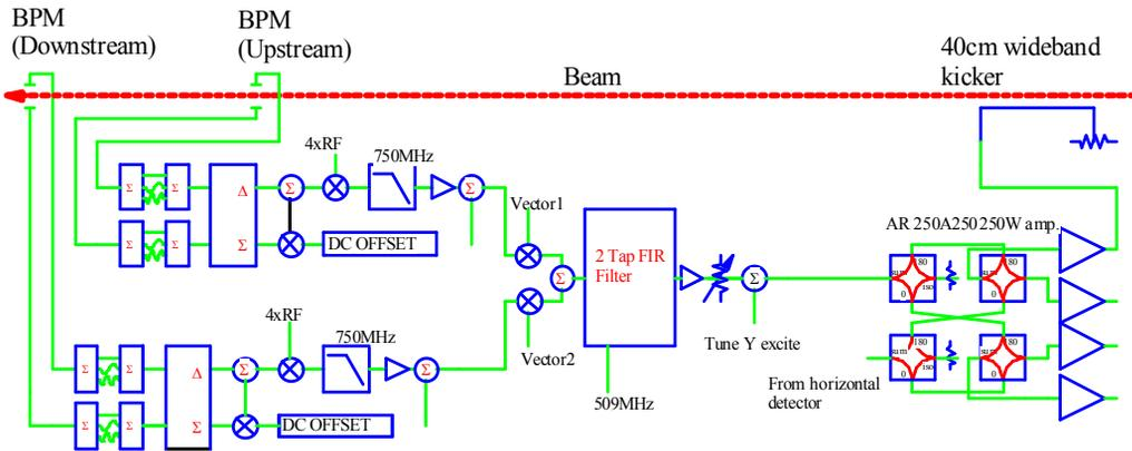
Figure 2: Block diagram of KEBB-LER transverse (vertical) feedback systems.
