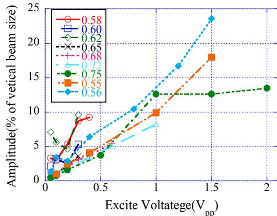
Figure 3: Measured vertical oscillation with externally supplied excitation amplitude.
