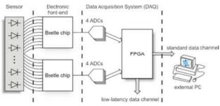
Figure 2: Proposed detector architecture.
