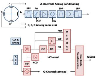
Figure 9: Key elements of the BPM read-out electronics.
