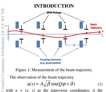
Figure 1: Measurement of the beam trajectory.
