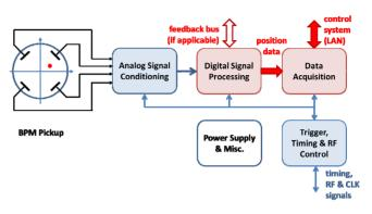
Figure 2: Schematics of a beam position monitor.
