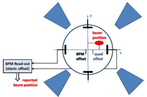
Figure 4: BPM and quadrupole offsets.
