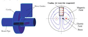
Figure 7: Waveguide-loaded cavity BPM.
