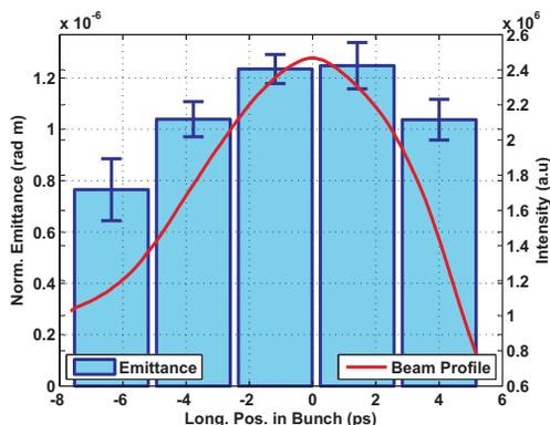
Figure 4: Measured slice emittances, series 6
