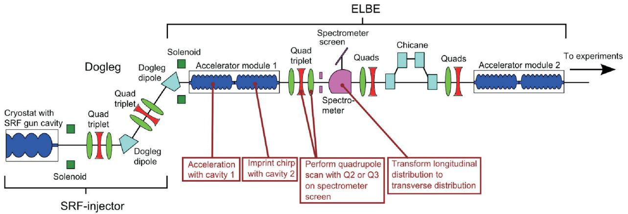
Figure 2: Schematics of ELBE beamline with SRF-injector and setup for slice emittance measurements
