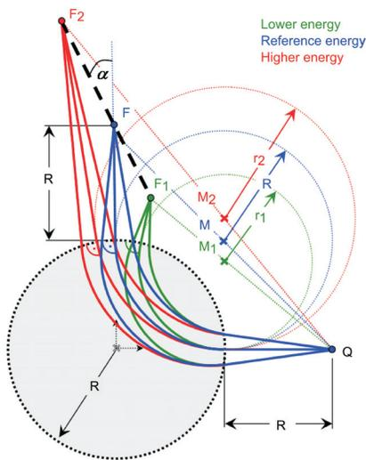
Figure 3: Imaging properties of the "Browne-Buechner" spectrometer
