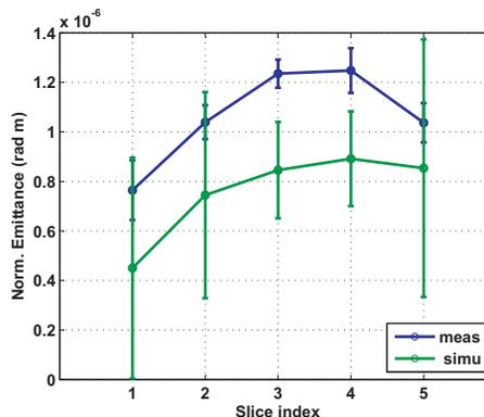
Figure 6: Comparison of slice emittance values determined from measurement and simulation, series 6
