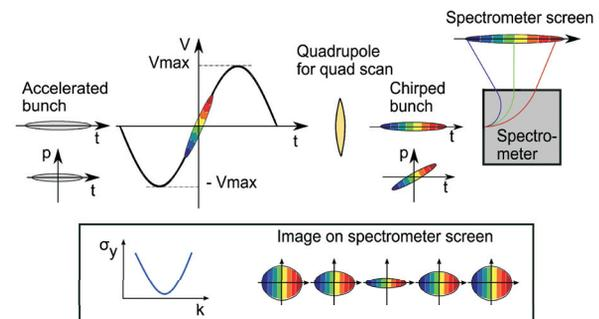
Figure 1: Working principle of the zero-phasing technique
