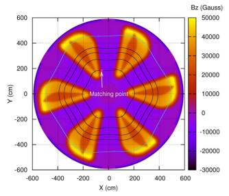
Figure 2: Plot of the closed orbits: the first closed orbit at injection which corresponds to an energy of 60 MeV/amu is shown in black, the next ones, still in black, correspond to a constant step size of energy of 80MeV/amu with respect to each other. The blue one however shows the closed orbit near the extraction, at 700 MeV/amu. The point marked with a pink color is the matching point inside the first closed orbit that will be used to match the beam properly.
