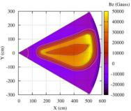
Figure 1: Plot of the z-component of the magnetic field in the median plane for one sector, with the isofield lines.
