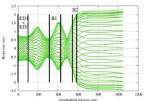
Figure 9: Radial beam envelope vs the longitudinal abscissa along the injection trajectory: there is almost no change in the beam envelope before and after applying the gradient to the dipole B2. However, the beam size exceeds 4 cm outside the pole gap which is fine especially that the radial inter-turn separation at the location of B2 is not limiting any more.
