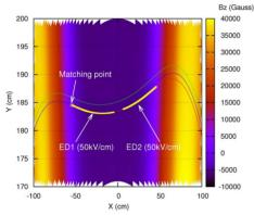
Figure 7: Plot of the beam trajectory inside the eletrostatic deflectors (red curve): the blue curve shows the first closed orbit (that has to be matched) while the green one represents the first accelerated orbit at the location of the septum.
