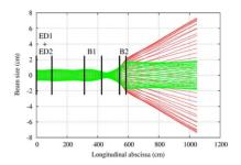
Figure 8: Axial beam envelope vs the longitudinal abscissa along the injection trajectory: the red curve shows the result when no gradient is introduced inside the magnet B2, while the green curve shows the result when a 0.68 kG/cm gradient is applied to the magnet B2. The difference between the two envelopes is observed after dipole magnet B2.
