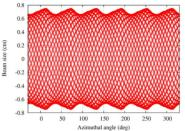
Figure 4: Axial beam envelope vs  $\theta$  along the 1st closed orbit.
