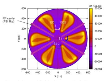
Figure 6: Layout of the injection system for the Superconducting Ring Cyclotron.
