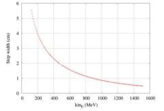
Figure 3: Plot of the transverse separation of the turns as a function of the kinetic energy: this result was obtained from tracking by searching for the closed orbits assuming **.BY-3.0** and by the respective authors a constant energy gain per turn of 4 MeV/amu.
