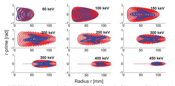
Figure 5: SIMION radial trace space plots for various (fixed) particle energies. Blue traces are Poincaré map in spiral AVF field, red traces in weak-focusing field. Note 4-lobed structure that reflects 4-sector geometry.
