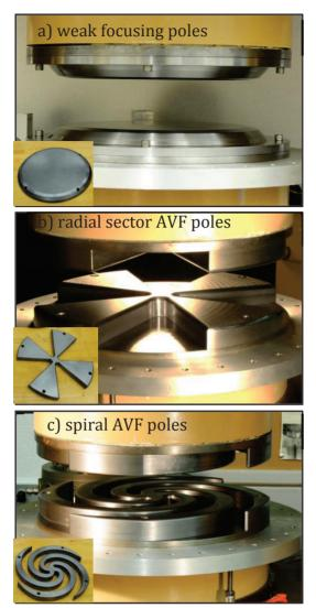
Figure 2: Rutgers cyclotron pole tips: a) weak focusing, b) radial sector, c) spiral AVF
