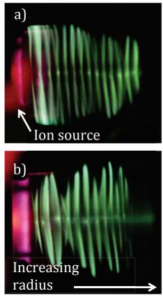
Figure 9: Betatron motion observed with radial Phosphor probe. a) weak focusing field, b) spiral AVF field, for DEE powered at 100 Watts.
