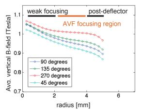
Figure 4: Average field profile over a circular path as a function of radius for several Archimedean spirals. Each spiral is defined by degrees swept from center to periphery. Note the weak focusing "bump" and flat
