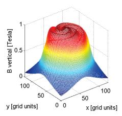
Figure 6: Spiral AVF measured field profile in midplane.
