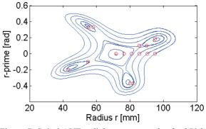
Figure 7: Spiral AVF radial trace space plot for 250 keV protons. Initial positions are marked in red. Note central orbit and 4 surrounding off-center fixed points.
