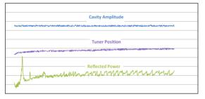
Figure 4: Initial one-hour stability test on a single resonator cyclotron (vertical axes are unscaled).
