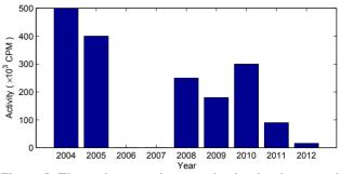
Figure 5: The cyclotron tank contamination level surveyed near the 1A foil position over the last several years (where the year 2006 and 2007's data were missing). It has been reduced by a factor of 5 to 10 in 2012.
