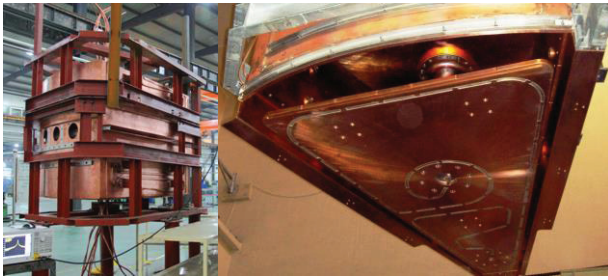
Figure 5: The installation (left) and the traces of multipacting (the darker colour on the cavity surface) at the ends of the cavity.
