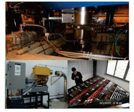
Figure 6: The installed dry pump and cryopumps (upper) and the cryopanel system (lower).
