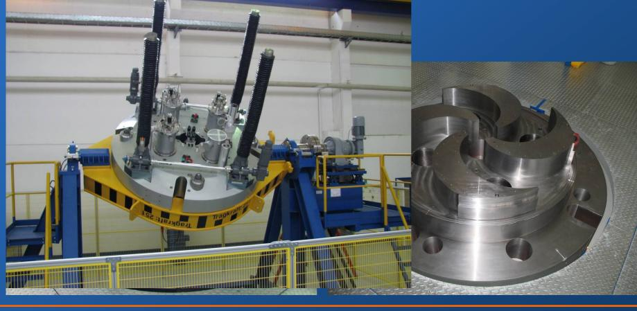
The VARIAN 250 MeV Superconducting Compact Proton Cyclotrons
