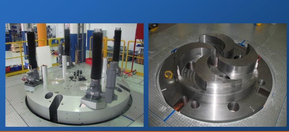
The VARIAN 250 MeV Superconducting Compact Proton Cyclotrons
