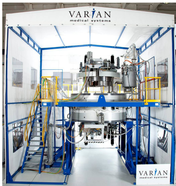
Figure 1: VMS-PT cyclotron no. 3 in a temperature stabilized cell (front cover removed for photo) during FATs
