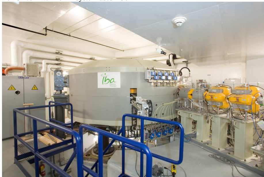
Figure 2. IBA 230 MeV resistive cyclotron for proton therapy
