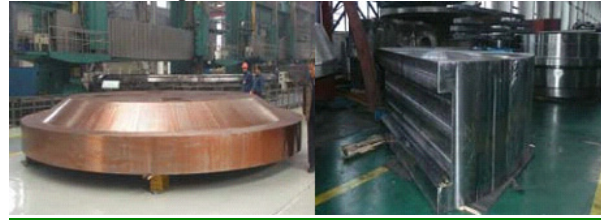
Fig. 3 One top yoke after pre-fine machining (left) and fabricated sector poles (right).
