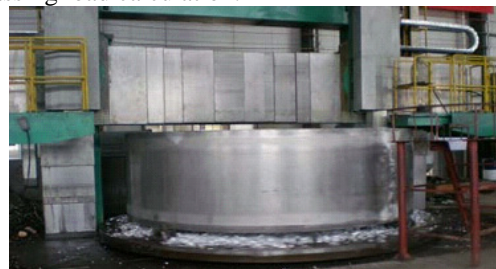
Fig. 10 The vacuum chamber in machining process.
