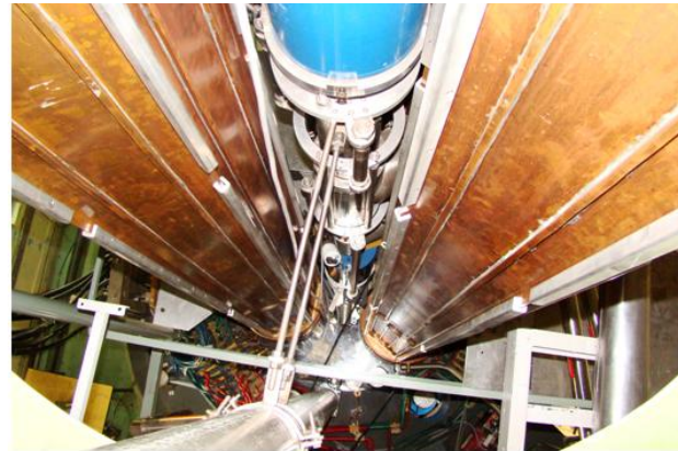
Figure 6: Vertical injection line on top of yoke
