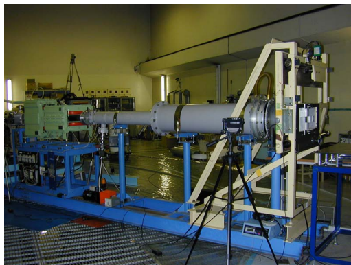
Figure 3: Beam course of C8 for physical experiments with wobbler magnets and scatterer to obtain uniform lateral distribution.
