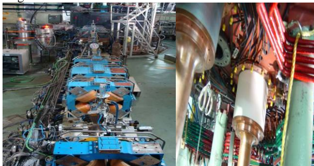
Figure 7a. Cyclotron with Zero degree Extraction Beam line, (7b) Coupling capacitor
