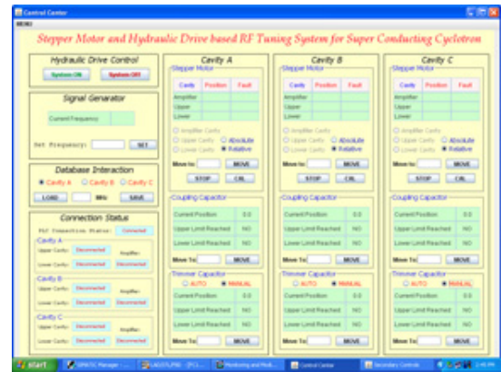
Figure 5: User Interface of the RF Tune operation control.
