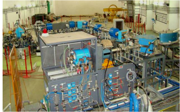
Figure 5: Installed ECR Ion Source and Injection Line
