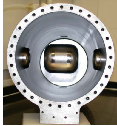
Fig. 4: Phase II cavity after etching.
