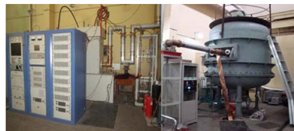
Fig. 15 High power RF cavity test stand.
