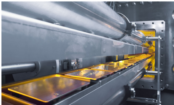
Figure 4: The phase probe structure, supporting the 21 fixed probes, during installation in a vacuum chamber of the SSC.
