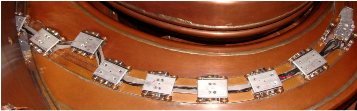
Figure 2: Main probe in derailed condition within the beam chamber.
