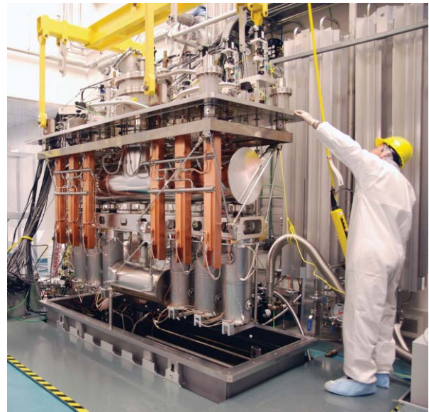
Fig. 6: Cryomodule SCC1 assembly prior to the first cold test
