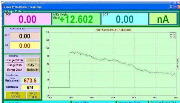
Figure 3: Current vs. radius for the Ne^{3+} beam
