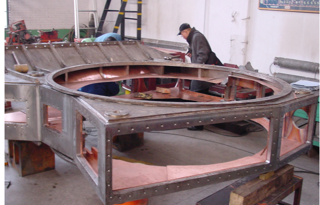
Figure 1: SFC double-deck vacuum chamber
