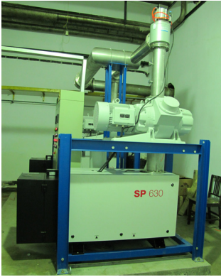
Figure 3: The new rough pumping stations of SSC and SFC
