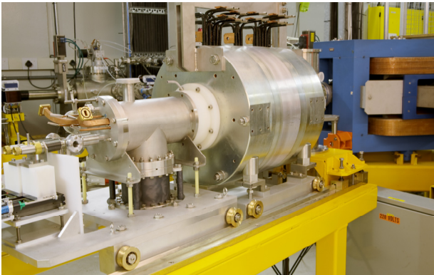
Figure 2: Partially assembled GTS2 ECRIS.
