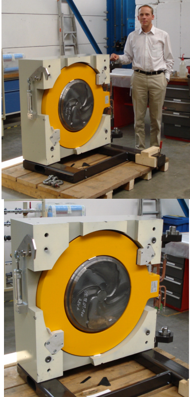
Figure 7: Cyclone® 3 being currently assembled at the Belgian IBA facility. One can distinguish the various vacuum chamber access in the return yoke: pumping and
