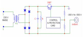
Fig-1: Schematic of Grid Power Supply
