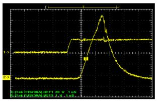
Figure 4: Crowbar measurement, Ch-1-Fault current & Ch-2 Trigger signal to Ignitron and time delay around 3 μs.
