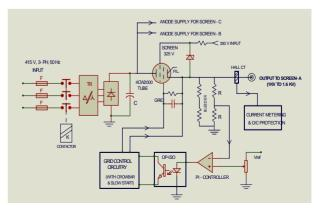
Figure 2: Schematic of Screen power supply.
