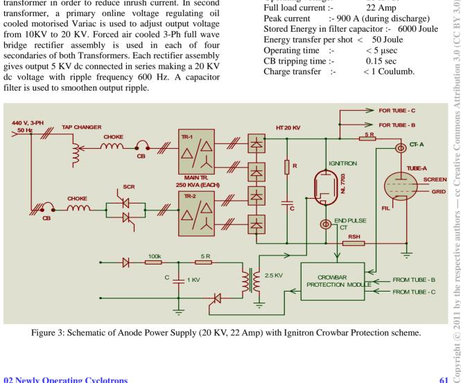
Figure 3: Schematic of Anode Power Supply (20 KV, 22 Amp) with Ignitron Crowbar Protection scheme.
