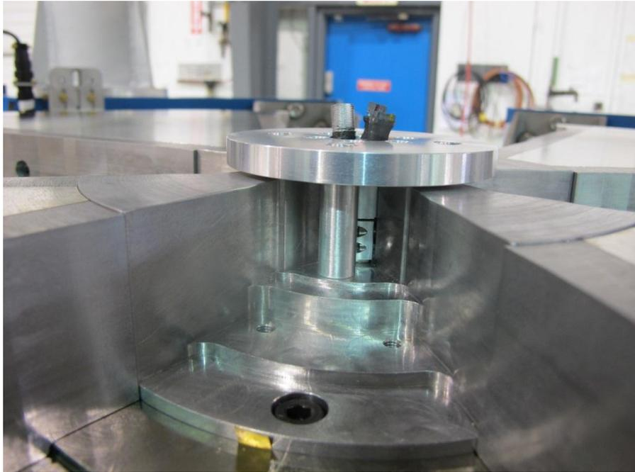
**Height Adjustment:** the HP arm template inserted into the main shaft of the mapper
