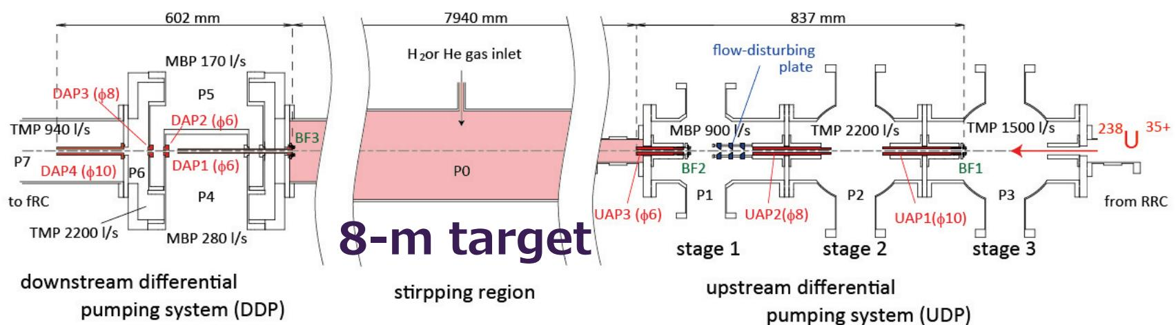
Gas was directly confined within **beamline** (H<sub>2</sub> 1 mg/cm<sup>2</sup>, He 3 mg/cm<sup>2</sup>)
