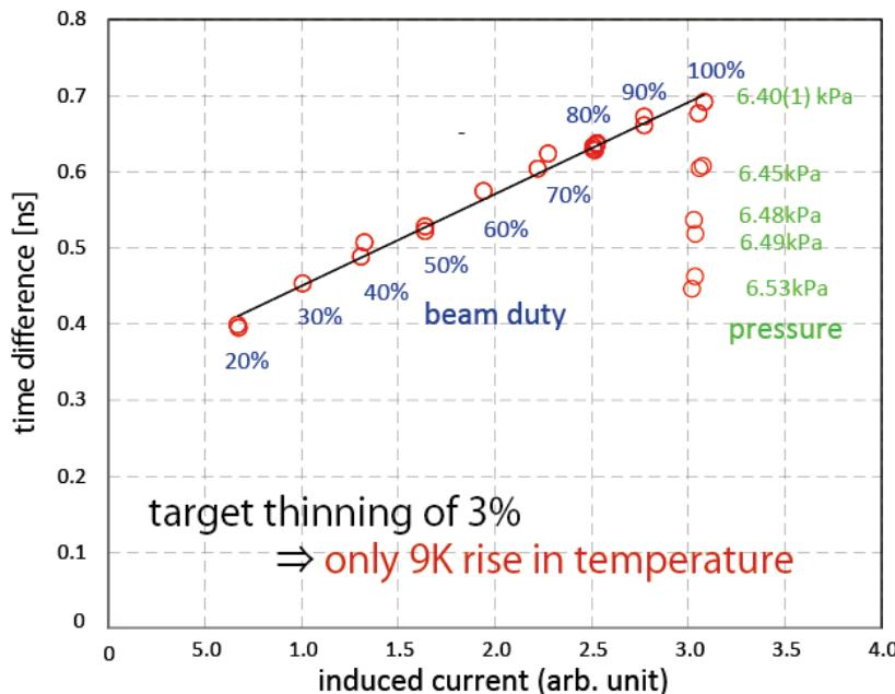
The TOF of  $\text{U}^{64+}$  beams as a function of the beam intensity using phase probes.
