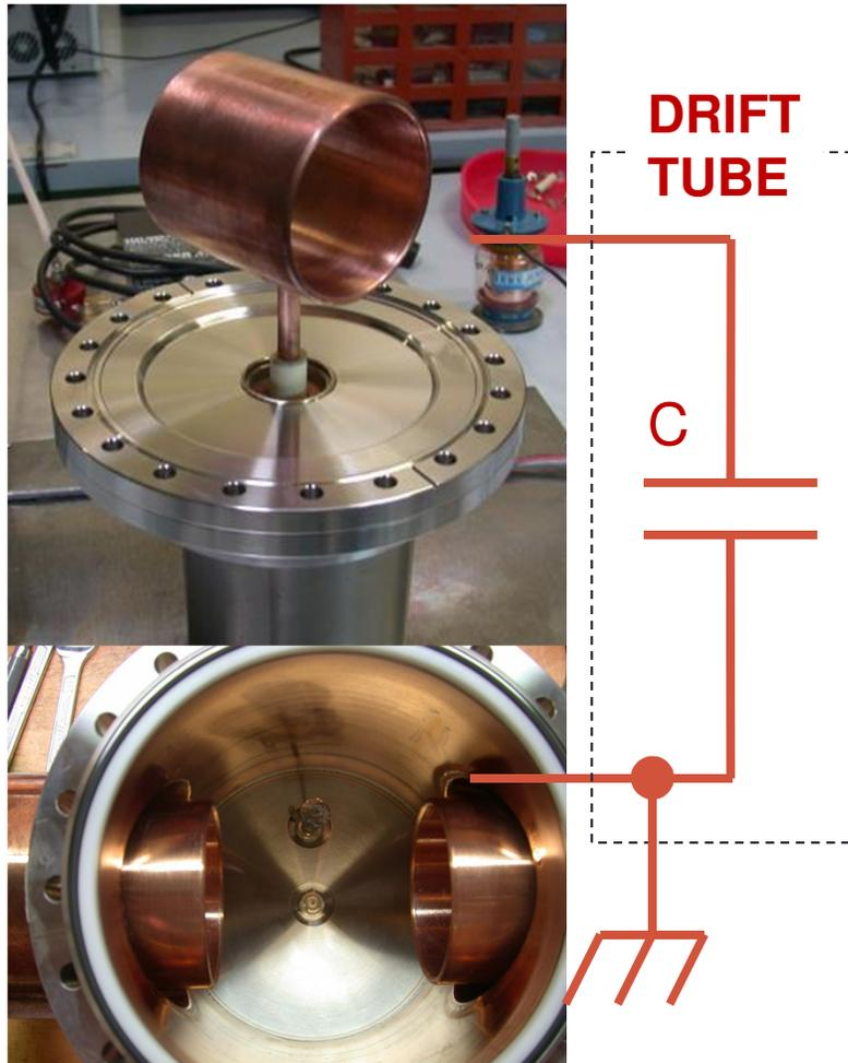
From the electrical point of view the **drift tube** can be seen as a **capacitance**.
