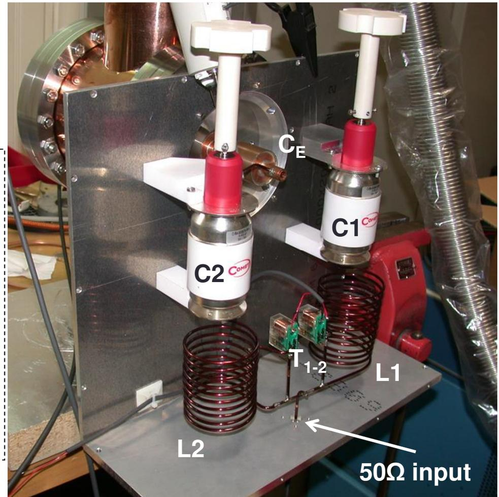
**Lower Bandwidth:** 13.3-25 MHz  $L_1 = L_2 = 4.2 \mu\text{H}$  ( $T_1$ - $T_2$  open)
