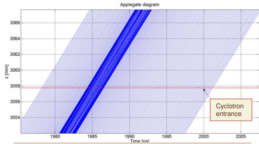
**Enlarged view of the Applegate diagram. There is the indication of the z-position of the Cyclotron entrance.**
