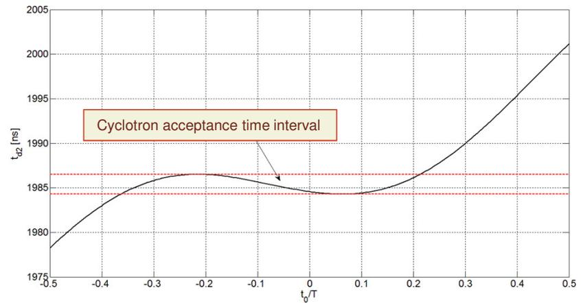
Arrival time of each particle at the Cyclotron entrance, with respect to the  $t_0$  time when each particle arrives at the  $z = 0$  position.  $T = 1/f$ .
