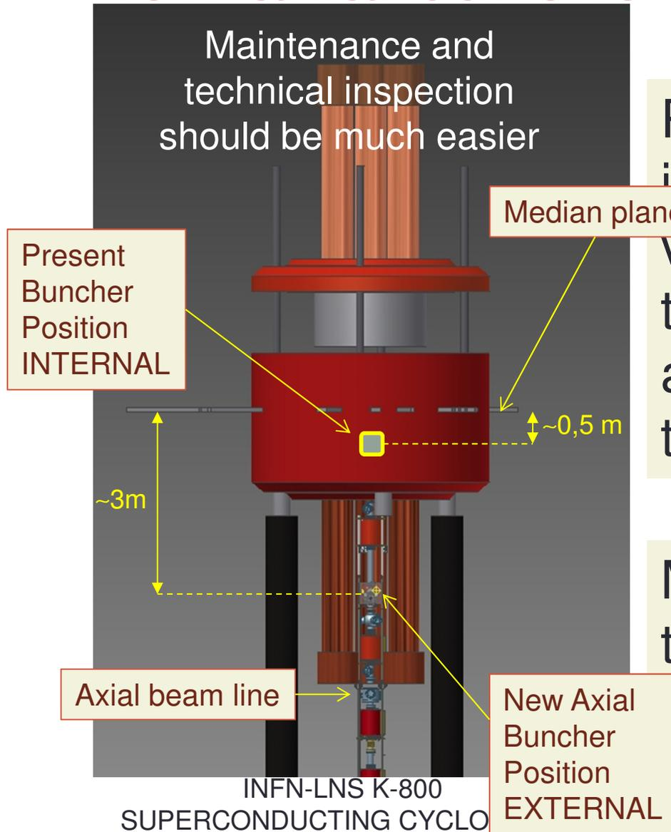
Present axial buncher is installed along the vertical beam line inside the yoke of the cyclotron at about half meter from the median plane.
