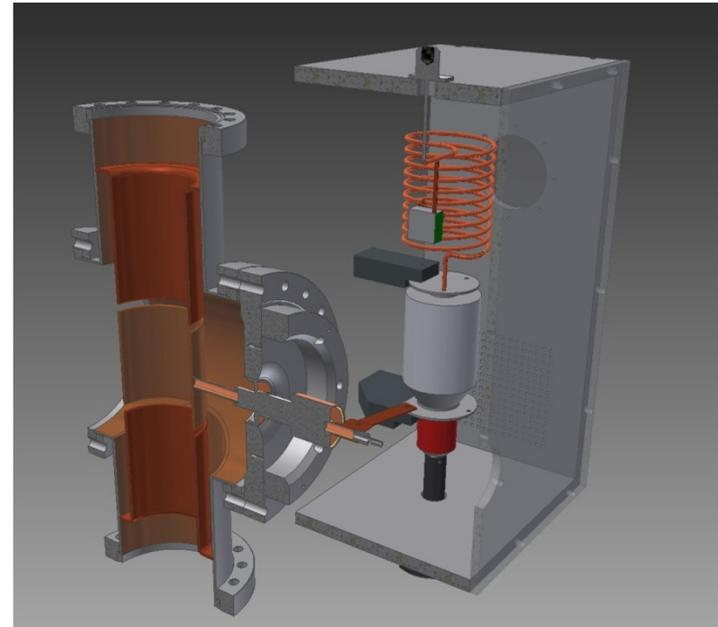
**This particular design prevents any connection through coaxial transmission line. It reduces the entire geometry, the connection losses, the total RF power and the maintenance.**
