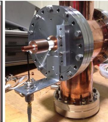
An LCR meter confirms the simulated capacitance value of **about 27pF** and, with a vector network analyser, the **self-resonance of 352,75 MHz** has been measured through an **N-adaptor**.
