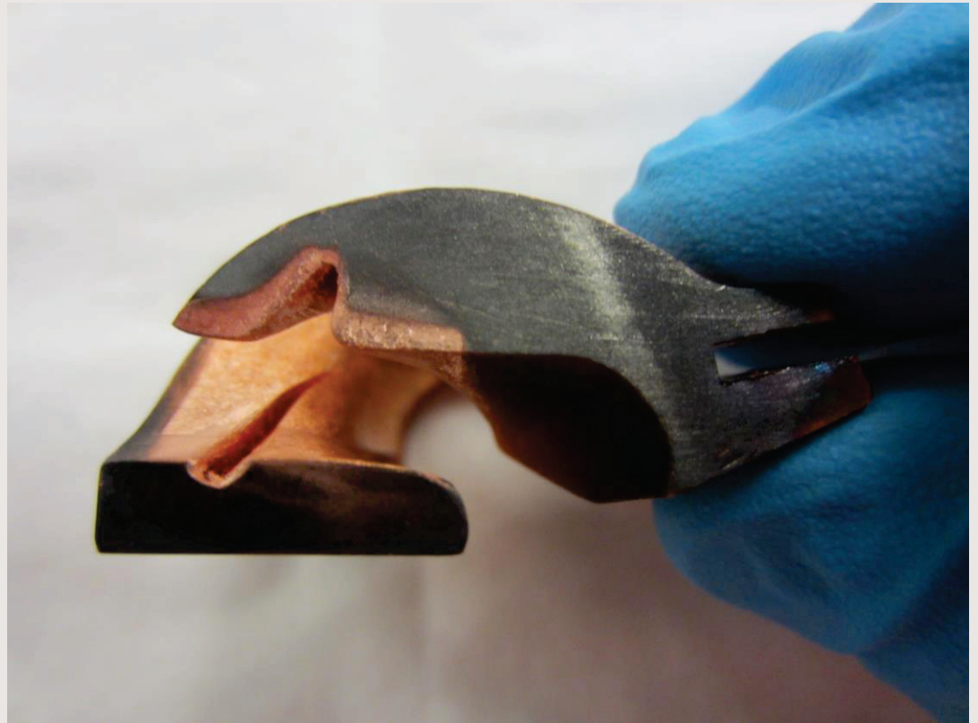
TR30-2 beam eroded inflector
