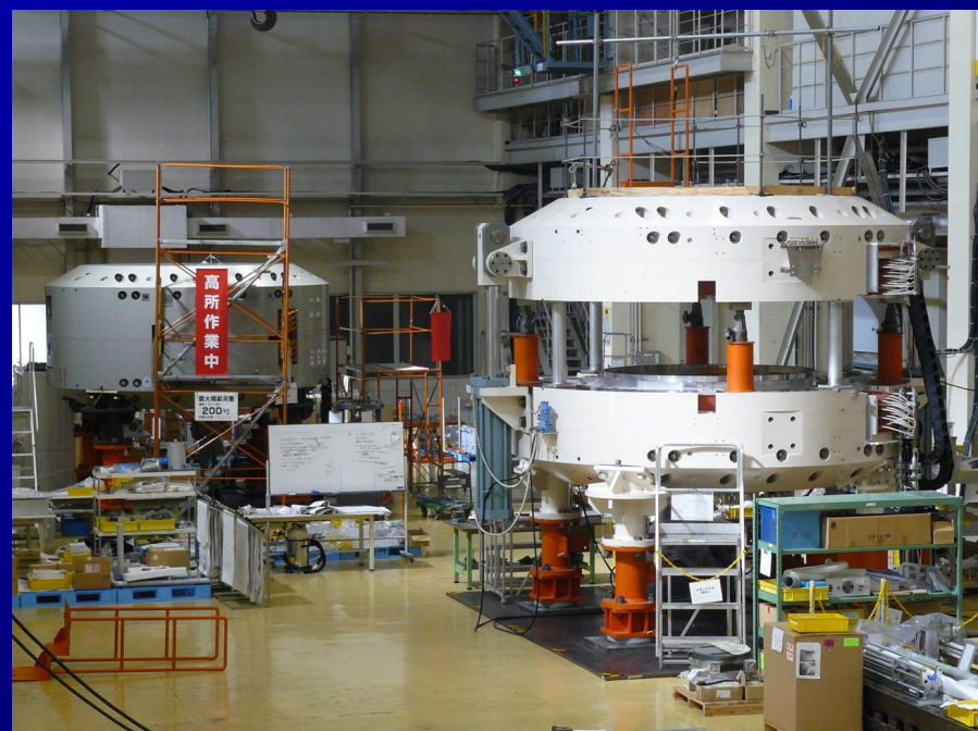
P235 cyclotrons manufactured and beam tested in Sumitomo Niihama Factory
