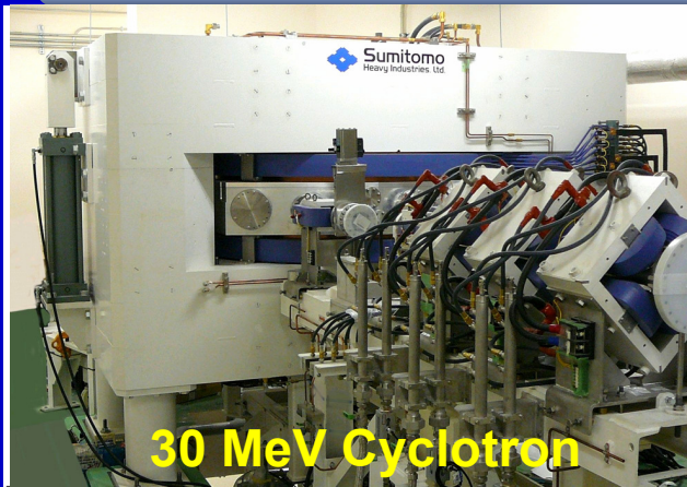
World First Cyclotron-based BNCT (Boron Neutron Capture Therapy)
