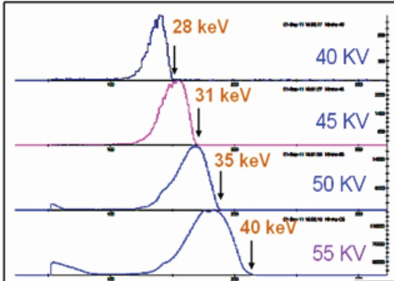
The **End point** has been “chosen” in the **linear** plot as the end of the “semi Gaussian” shape.
