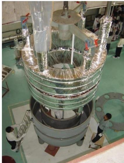
Multilayer Insulation and vacuum chamber
