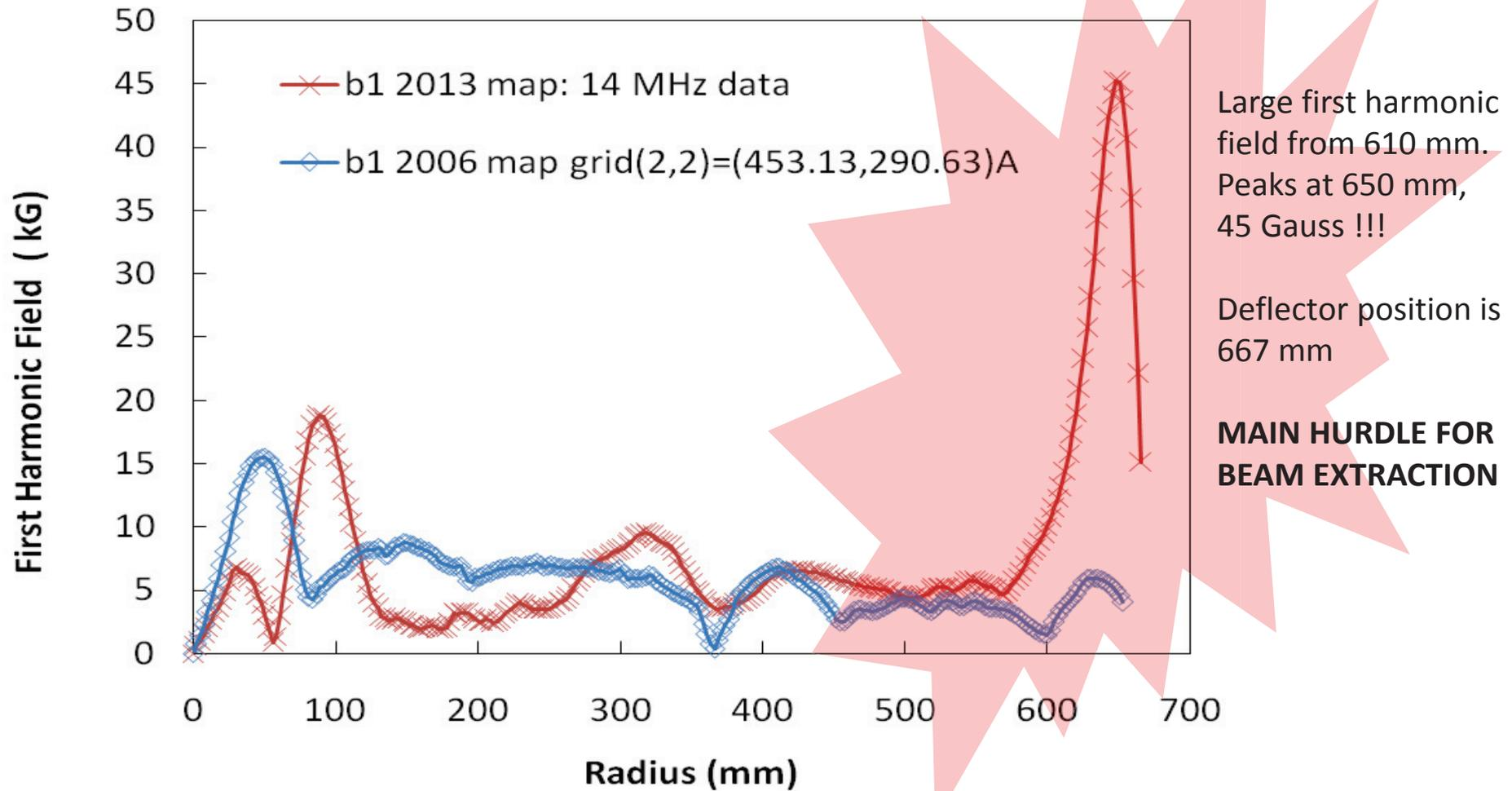
Large first harmonic field from 610 mm. Peaks at 650 mm, 45 Gauss !!!
