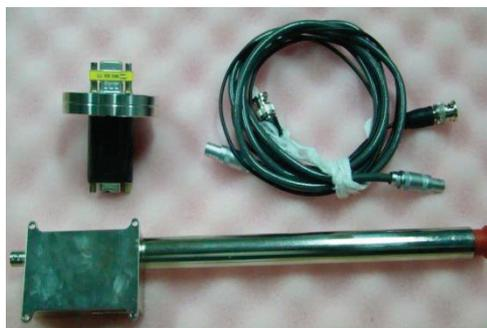
X-RAY DETECTOR WITH ITS FEED THROUGH AND CABLINGS
