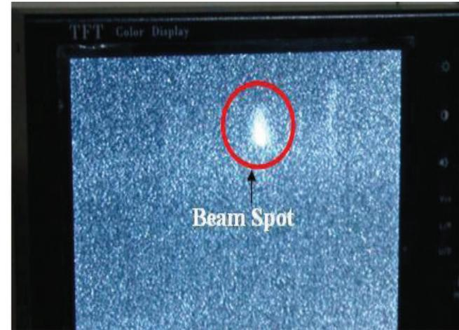
Accelerated Ne<sup>3+</sup> Beam on viewer probe
