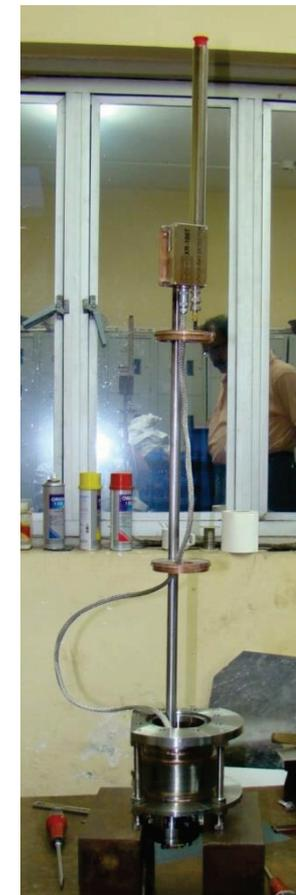
X-RAY DETECTOR ON ITS HOLDING SETUP
