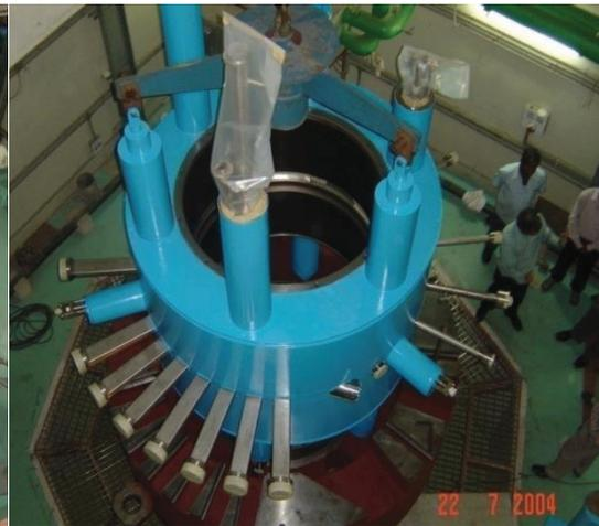
Cryostat with Median plane inserts
