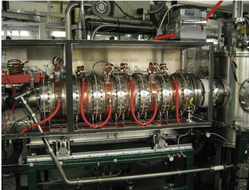
120 cm gas catcher from Argonne National Lab operates with helium at  $\sim 100$  mbar and  $-5^\circ\text{C}$
