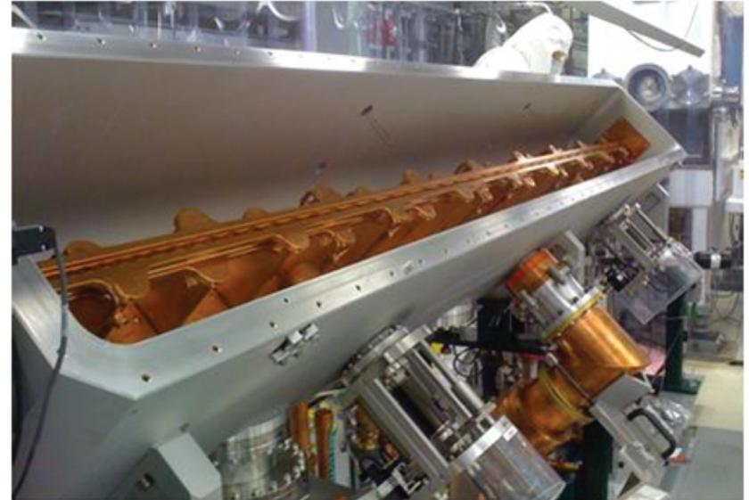
Quadrupole transport channel with longitudinal modulation to achieve accelerating field along the beam direction
