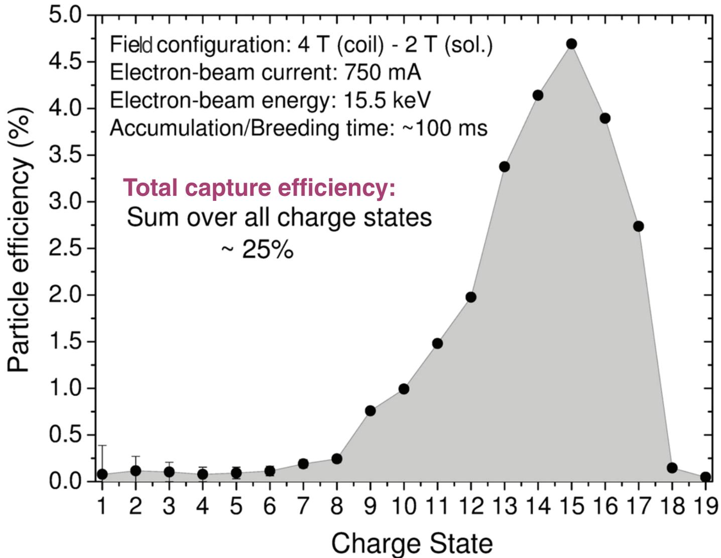
**Total capture efficiency is in good agreement with expected capture efficiency (~30%) for an electron beam current density of ~350 A/cm<sup>2</sup>**
