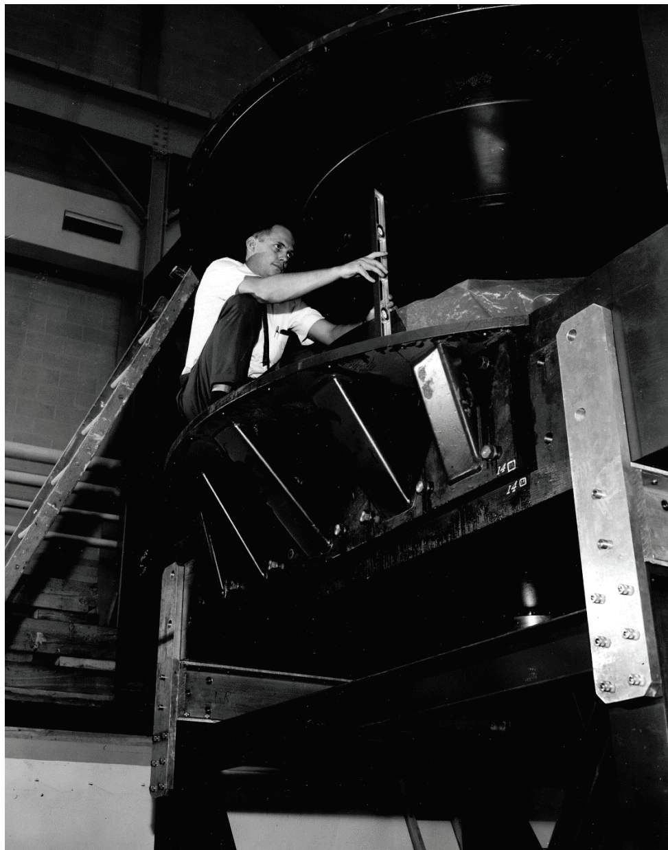
Checking alignment of the K50 Cyclotron
