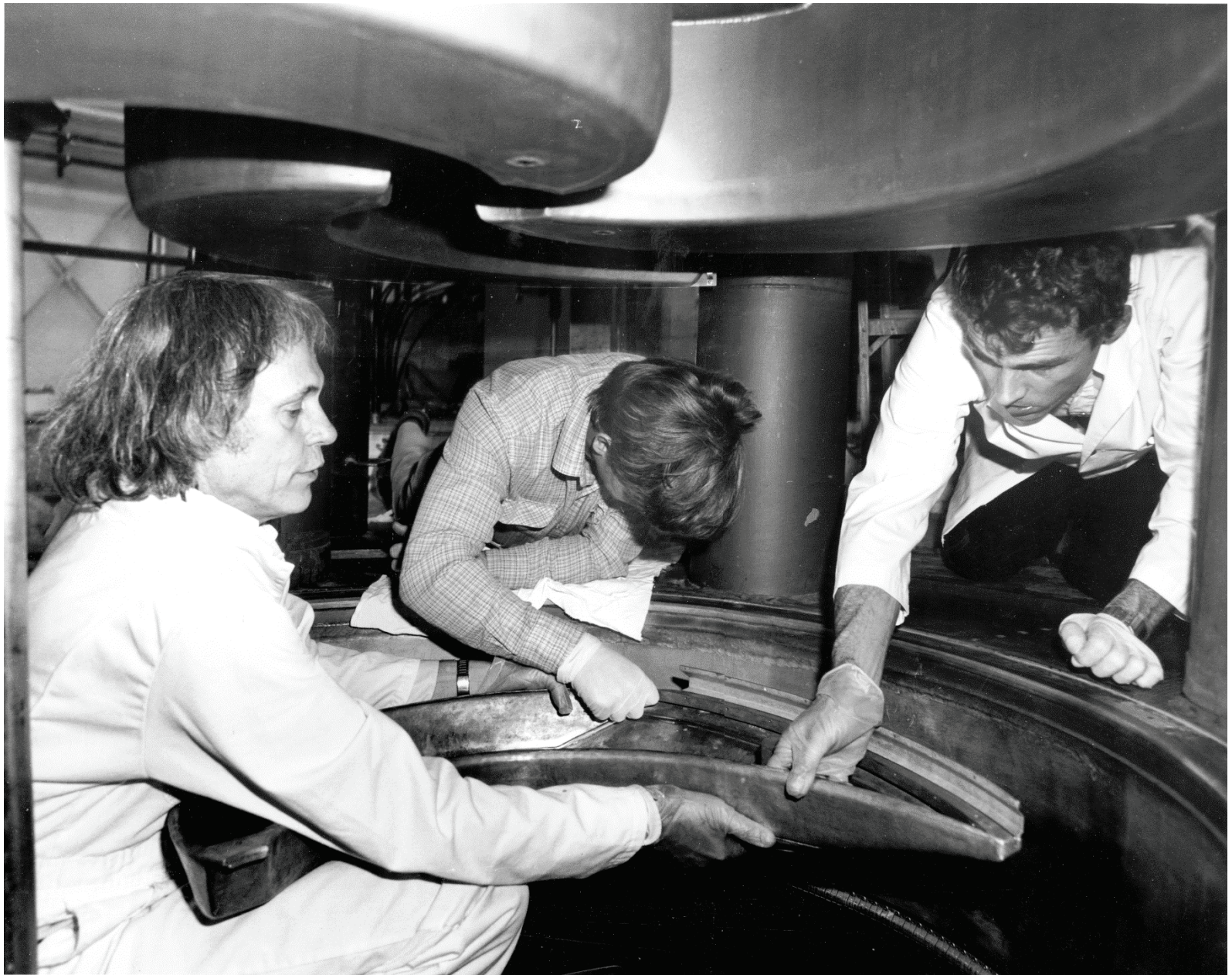
Inside the K500 cyclotron beam chamber adjusting the dees,
