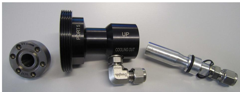
New conical design<sup>#</sup>: Niobium insert, target body, one piece water diffuser
