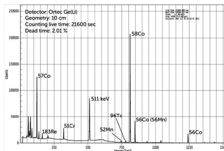
Figure 5: radionuclidic impurities in <sup>18</sup>F-solution (Conical 8)
