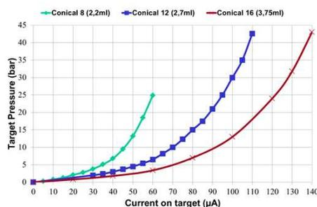
Figure 4: target pressure curves for given filling volumes
