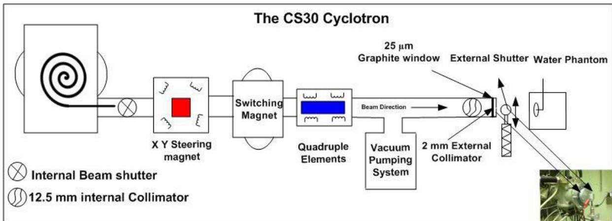
Figure 2: Beam controller components along the beamline 2.
