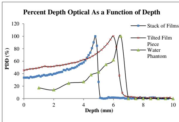
Figure 4: The PDDs of the two film measurements (stacked film pieces and tilted film piece) and the water phantom as a function of depth with CSD of 70 cm.
