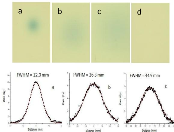
Figure 3: Scans and vertical profiles of the irradiated HD-V2 film pieces when placed at a) 40, b) 70 and c) 100 cm from the aperture d) background film.
