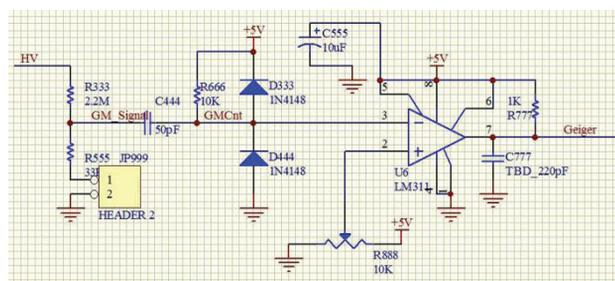
Figure 3: The electronic design for converting the gamma rays to a measurable electrical pulse.
