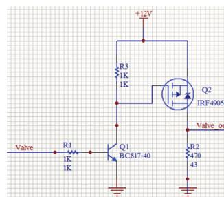
Figure 2: A driver for relating valves and microcontroller to each other.
