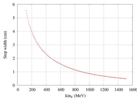
Figure 3: Plot of the transverse separation of the turns as a function of the kinetic energy: this result was obtained from tracking by searching for the closed orbits assuming a constant energy gain per turn of 4 MeV/amu.
