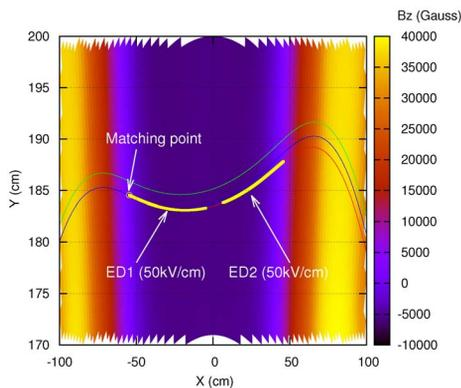
Figure 7: Plot of the beam trajectory inside the electrostatic deflectors (red curve): the blue curve shows the first closed orbit (that has to be matched) while the green one represents the first accelerated orbit at the location of the septum.
