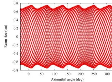
Figure 4: Axial beam envelope vs  $\theta$  along the 1st closed orbit.
