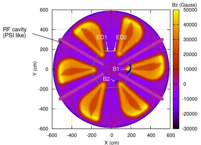
Figure 6: Layout of the injection system for the Superconducting Ring Cyclotron.
