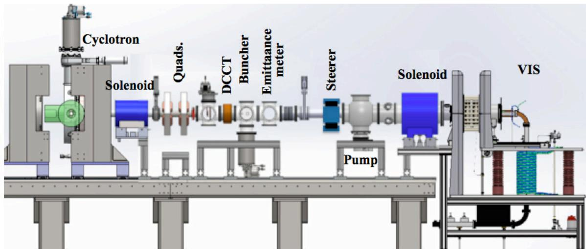
Figure 1: Layout of the test stand at the BCSI development lab in Vancouver, Canada. The ion source is in a high-voltage cage (not shown) at far right; the test cyclotron is on the left. Total length of the test stand is about 5 meters.
