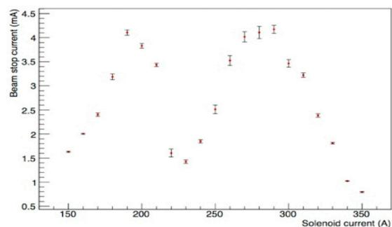
Figure 2: Beam stop current vs. solenoid current. The beam current is detected on beam stop behind a  $\phi=20$  mm collimator. Protons peak at 190 A,  $H_2^+$  at 280 A. Extraction voltage was lowered to 40 kV to better match the range of solenoid current.
