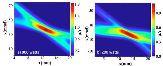
Figure 4: Emittance plots for combined  $H_2^+$  and protons, a) at 900 watts microwave power, b) for 200 watts.
