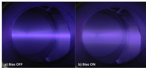
Figure 3: a) Beam profile 50 cm upstream of collimator with bias OFF. b) beam profile with bias ON.
