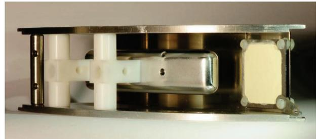
Figure 5: Electrostatic deflector assembly.
