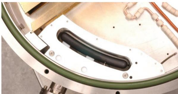
Figure 7: Deflector assembly, with clearance slot exposing electrode, now coated with Aerodag-G.
