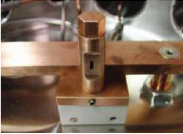
Figure 3: The Ion Source stuck under the dummy-dee.
