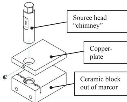
Figure 2: The basic setup of our ion source.
