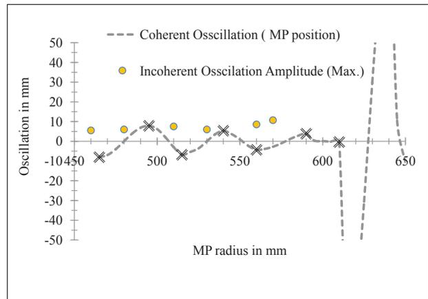
Figure 3: Radial betatron oscillation obtained from shadow measurement.
