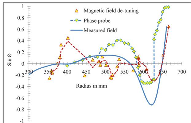
Figure 4: Particle phase history measured with two different methods.
