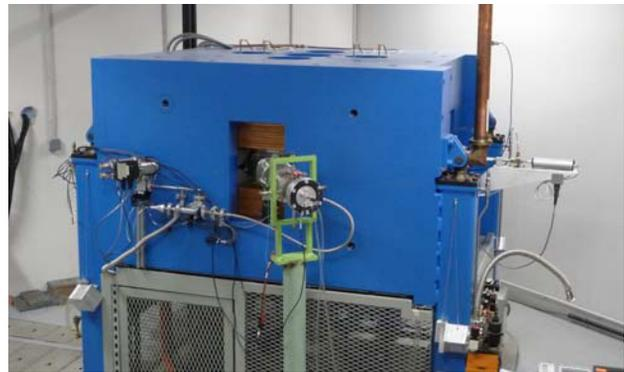
Figure 1: Picture of the TR24 cyclotron installed at IPHC in Strasbourg. The water cooled beam dump provided by ACSI is visible at the end of the beam pipe.
